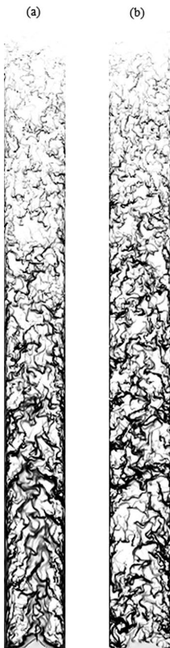
Figure 2. Snapshots of the particle phase volume fraction field extracted from the 2D simulation of the kinetic theory model equations in a 2D domain with partial slip (Johnson and Jackson 45 ) BC with (a) \phi = 0.0001 and (b) \phi = 0.6 for the particle phase and free slip BC for the gas phase at all walls.
